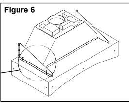
**Step 7:** Using help if necessary, lift the liner, Blower and mounting bracket assembly into position and hang on the screws extending from the mounting plate. Make sure the brackets are firmly seated into the key hole slot and then tighten all the screws (See figure 7).
