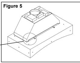
Step 6: Fasten the Metal Mounting brackets to the liner with 4 each 10-24 x 3/4" screws and nuts. Figure 0 for the liner these at this time (See figure 6).
