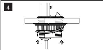
Place locking ring into collar. Identify and align arrows on the collar and locking ring to ensure the thread is engaged properly. Turn the locking ring clockwise to tighten. Make sure rubber washer is compressed tightly on underside of surface. Tighten the screw until ring firmly grips the surface.
