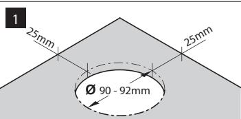
Cut out 90-92mm Diameter hole in work surface. Allow minimum 25mm clearance around the cut hole. When choosing location, select a surface between 10mm and 50mm thick.
