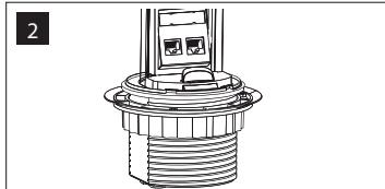
The locking ring with rubber washer is supplied in the packaging. If attached to the mounting collar, remove it by rotating it in a counter-clockwise direction prior to lowering the unit into its final location.
